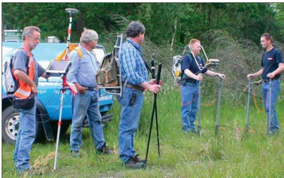
Gasunie deploys indirect inspection teams to conduct DC voltage gradient and close-interval potential surveys, as well as acquire GPS measurements for any defect indications. Indirect inspection seeks to identify and define the severity of coating faults and other anomalies where corrosion activity may be occurring. NACE requires at least two such inspections over the entire length on an ECDA region (Fig. 3).
