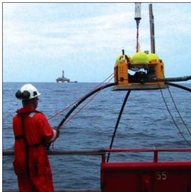
Long dipole receiver is deployed from an acquisition vessel at the start of a controlled source electromagnetic survey. Photo courtesy of Offshore Hydrocarbon Mapping PLC.
